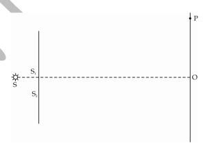
The figure, drawn here, shows a modified Young's double slit experimental set up. If SS<sub>2</sub> SS<sub>1</sub>, =  $\lambda/4$ ,
